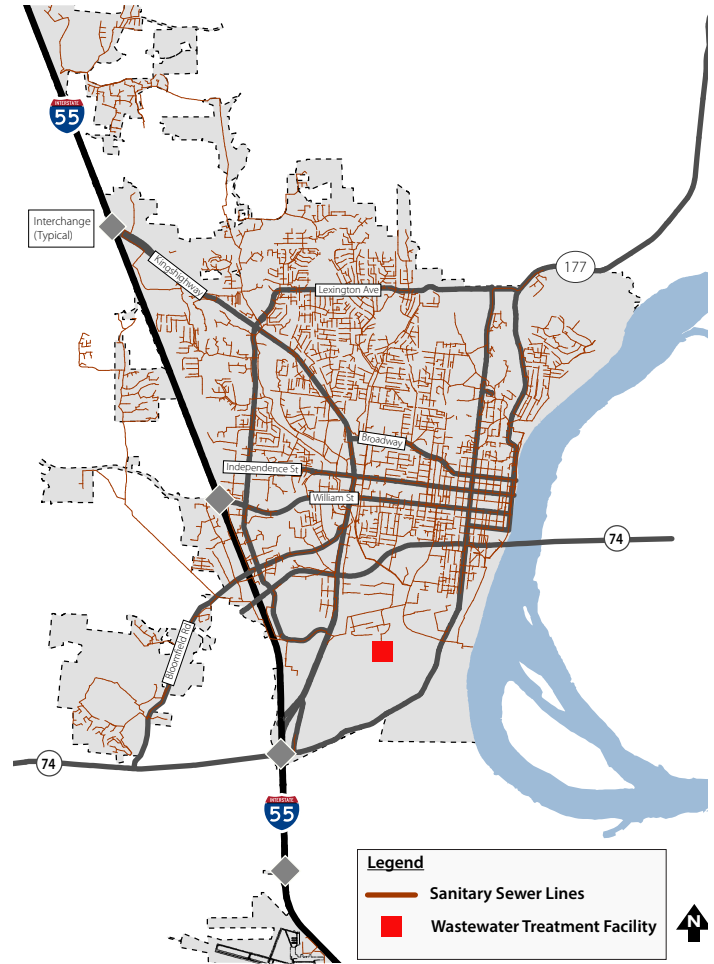
Figure 6.2 | Wastewater System Map
